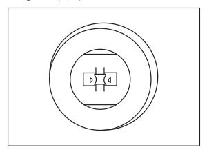
Access sign raceway/wiring box, and cut all ballast input and output wires as shown. Do not remove ballast if removal leaves opening in raceway.
