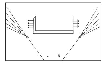
**6.** Insert Keystone Sign Hero LED tubes and rotate to desired position for optimal illumination. Ensure side marked "L" is connected to corresponding line socket and "N" is connected to corresponding neutral socket.
