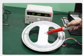
Testing whether the withstand voltage is within the specified value, to avoid sudden voltage surges such as short circuit, operation error, fault, etc, causing breakdown or accidents.
