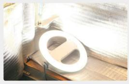
The test time is about 720 hours. After test the lamp working regularly, no discoloration appearance, no yellowing of the PC lens.
