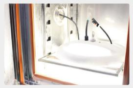
The test equipment opening 4hours, keeping temperature<-40 °C the lamp working fine. The test equipment opening 4hours keeping temperature>60 °C, the lamp keep working fine.
