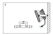
3. Drill 2x hole as Fig.2, the distance can be 91~140mm, fixing \$00 expansion screws and bracket on the wall.
