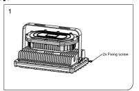
1. Take the fixture and accessory out from cartoon box, tighten 2x angle holder screw as Fig.1.
