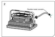
2. Through the cable to flexible metal conduit and tighten it with the fixture.
