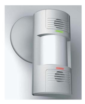
The LOS-WDT Series wall-mount dual-technology sensors are used to control lighting in spaces that have pendant fixtures, ceiling fans, or high ceilings (more than 12 ft./ 3.7 m), where ceiling-mount occupant sensors would not function reliably. The adaptive technology eliminates manual sensitivity and timer adjustments during installation and over the life of the product.
